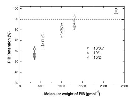
**Figure 13**: PIB retention by the PAN/ PDMS composite membranes prepared at pre-polymer/cross-linker of various ratios as a function of the molecular weight of PIB. Experimental conditions: feed concentration of 8 %(w/w),  $\Delta p=7$  bar, at 24  $\pm$  3 °C.
