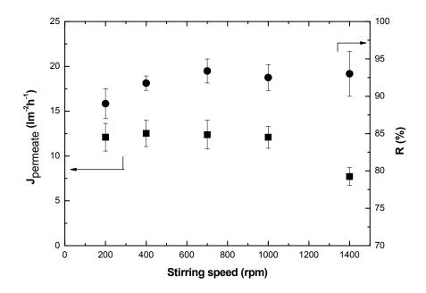
*Figure I.1:* The permeate flux and membrane retention for the feed solution of 8 % (w/w) oil/hexane. Experimental conditions: 7 bar,  $24 \pm 3$  °C.
