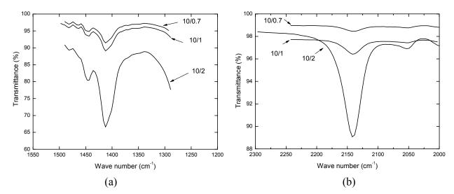
*Figure 4:* ATR-FTIR spectra of the dense PDMS membrane prepared at prepolymer/cross-linker of various ratios for (a) vinyl group (b) SiH group, respectively.
