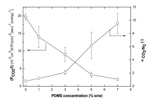
**Figure** 7: The normalized CO<sub>2</sub> permeability ( $P_{CO2}/l$ ) and  $\alpha_{CO_2/N_2}$  of the composite membranes as a function of the PDMS concentration in the coating solution. Experiments performed with pure gas at  $24 \pm 3$  °C.
