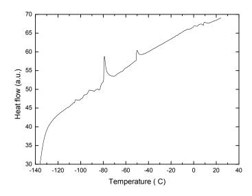
Figure 5: Heating curve of a dense PEO-PDMS-PEO membrane.
