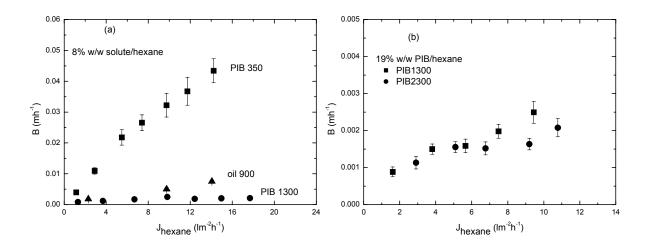
*Figure 12: Effect of molecular weight at (a) low feed concentration and (b) at high feed concentration upon oil permeability.*
