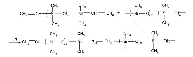
*Figure 1*: Scheme of the cross-linking reaction for the silicone network formation.
