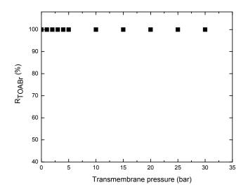
*Figure 11:* TOABr retention by the PAN/PDMS composite membrane as a function of transmembrane pressure, for 8 and 20% w/w TOABr/toluene solutions.
