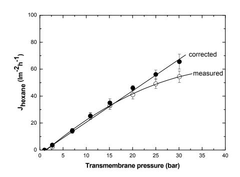
**Figure 6**: Hexane flux as a function of transmembrane pressure: measured and corrected data for the concentration mode. Experimental conditions: 0.008 mol fraction oil/hexane feed, at  $24 \pm 3$  °C.
