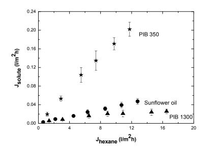
*Figure* 7: Solute flux as a function of the hexane flux for solutes of various MW. Feed concentration: 8 % (w/w).
