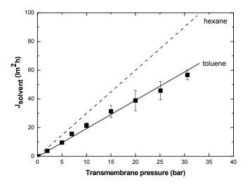
*Figure 5*: Toluene and hexane flux through PAN/PDMS composite membrane as a function of transmembrane pressure, at  $24 \pm 3$  °C.
