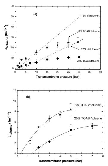
*Figure 10:* (a) Toluene flux as a function of transmembrane pressure at various TOABr/toluene concentrations, at  $24 \pm 3 \,^{\circ}$ , and (b) zooming in at low-pressure range.
