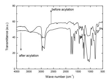
*Figure 2:* FTIR spectra of the PEO-PDMS-PEO copolymer before and after acylation.
