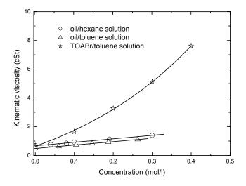
Figure 2: Kinematic viscosity of the feed solutions used in this study.
