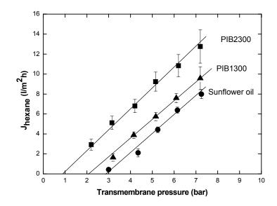
*Figure 5*: *Hexane flux as a function of transmembrane pressure for various solute/hexane systems. Feed concentration: 19 % (w/w).*
