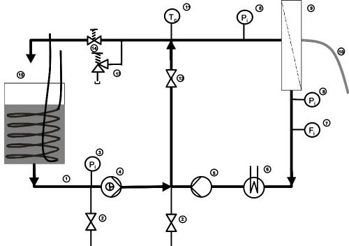
1=feed line, 2=drain, 3=vacuum pressure meter, 4=frequency controlled pressure pump, 5=frequency controlled circulation pump, 6=heat exchanger, 7=flow meter, 8=pressure meters, 9=membrane module, 10=permeate tubing, 11=temperature controller, 12=ball valve, 13=pressure relief valve, 14=backpressure valve, 15=feed vessel.
