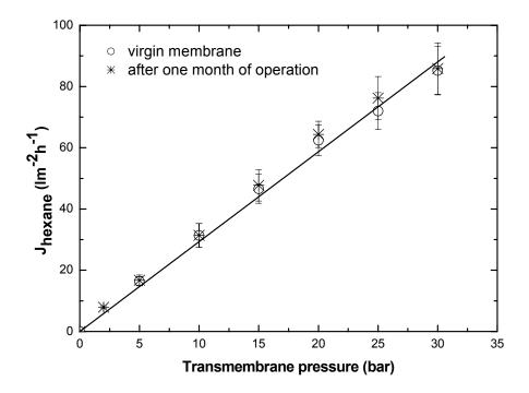
**Figure 4:** Hexane flux as a function of transmembrane pressure through a *PAN/PDMS* virgin membrane and through one and the same membrane after about 1 month of oil/hexane permeation experiments, at  $24 \pm 3$ °C.
