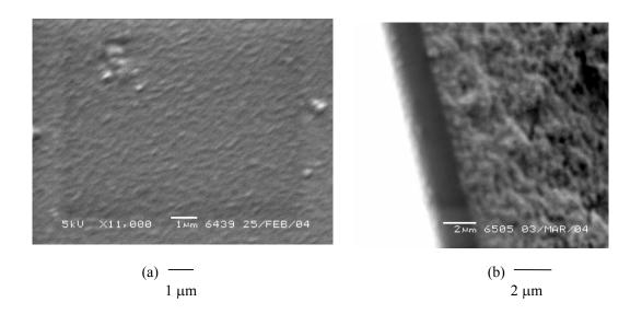
*Figure 14: SEM pictures of (a) the top-surface and (b) the cross-section of the GKSS membrane.*
