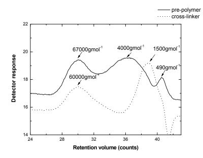
*Figure 2*: The molecular weight of the PDMS pre-polymer and cross-linker determined by GPC.
