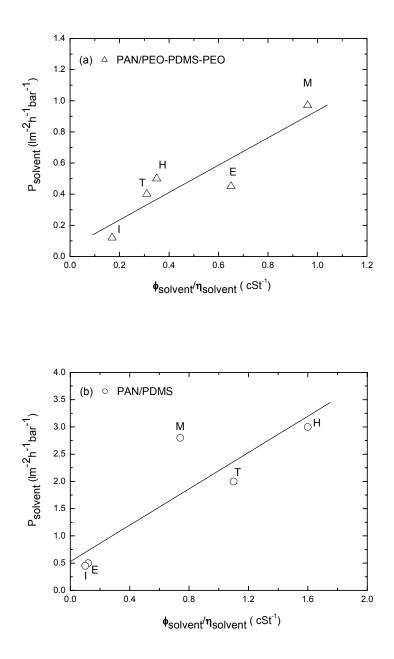
**Figure 6:** Solvent permeability measured at 30 bar through (a) PAN/PEO-PDMS-PEO and (b) PAN/PDMS membrane as a function of membrane swelling ( $\phi_{solvent}$ ) and solvent viscosity ( $\eta_{solvent}$ ). I, E, M, T, H stands for isopropanol, ethanol, MEK, toluene, and hexane, respectively.
