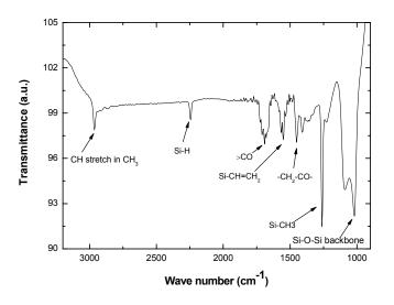
Figure 13: ATR- FTIR spectrum of the MPF-50 membrane.
