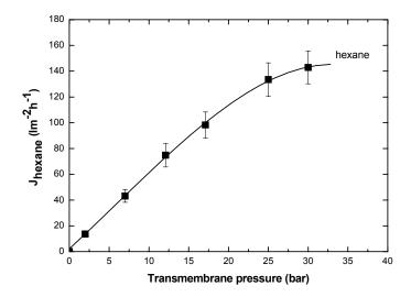
*Figure 13:* Hexane flux through the GKSS membrane as a function of transmembrane pressure at  $24 \pm 3$  °C.
