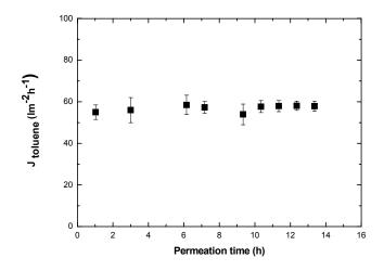
*Figure 4*: Toluene flux through PAN/PDMS composite membrane as a function of permeating time, at 30 bar and  $24 \pm 3$  °C.
