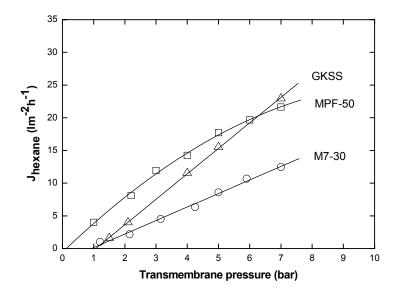
*Figure 16*: *Hexane fluxes as a function of the transmembrane pressure. Experimental conditions:* 8 % (*w/w*) *oil/hexane feed solution, at*  $24 \pm 3$  °C.
