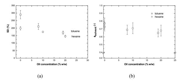
*Figure 3: Typical results of the effect of the oil concentration upon (a) swelling degree of PDMS dense membranes and (b) solvent fraction, at various oil concentrations.*
