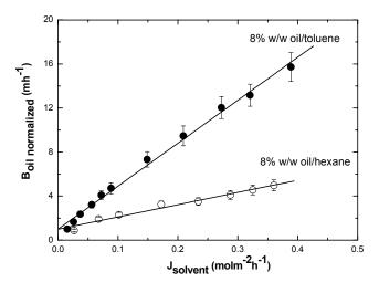
*Figure 8*: Effect of  $J_{solvent}$  upon normalized oil permeability coefficient, for 8 % w/w oil/toluene and oil/hexane concentration.
