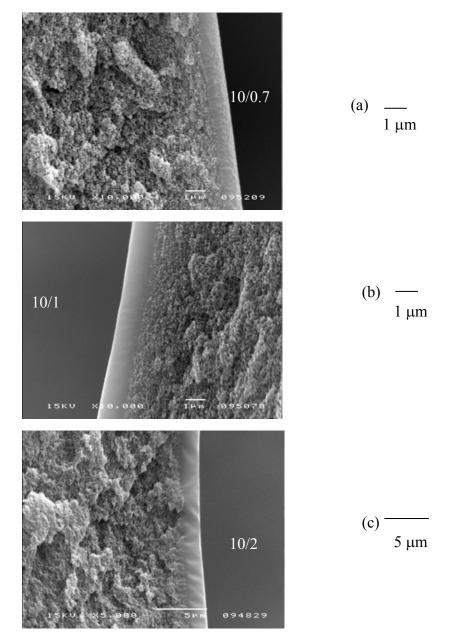
**Figure 10**: SEM pictures of the cross-section of PAN/PDMS composite membranes prepared at pre-polymer/cross-linker ratio of (a) 10/0.7 (magnification 10000x), (b) 10/1 (magnification 10000x) and (c) 10/2 (magnification 5000x).
