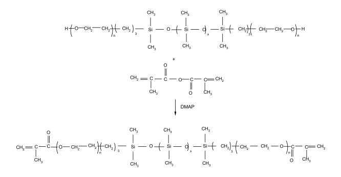
Figure 1: Synthesis of a UV-curable PEO-PDMS-PEO copolymer.
