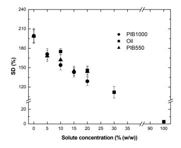
*Figure 2: Typical results of the effect of the solution concentration upon the swelling degree of PDMS dense membranes, for various solute/hexane systems.*
