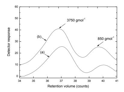
*Figure 4*: *MW of the PEO-PDMS-PEO copolymer determined by GPC (a) before and (b) after acylation.*
