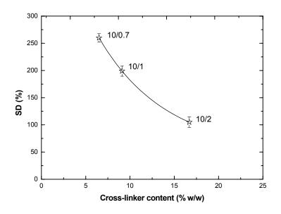
*Figure 5*: The effect of the cross-linker content upon the swelling degree (SD) of PDMS dense membranes in hexane.
