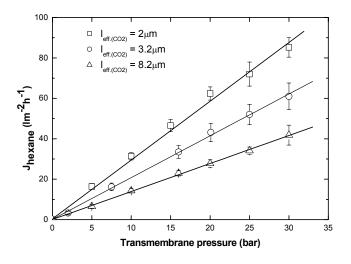
*Figure II.2:* Hexane flux as a function of transmembrane pressure through *PAN/PDMS* of various thicknesses, at  $24 \pm 3 \,^{\circ}$ C.
