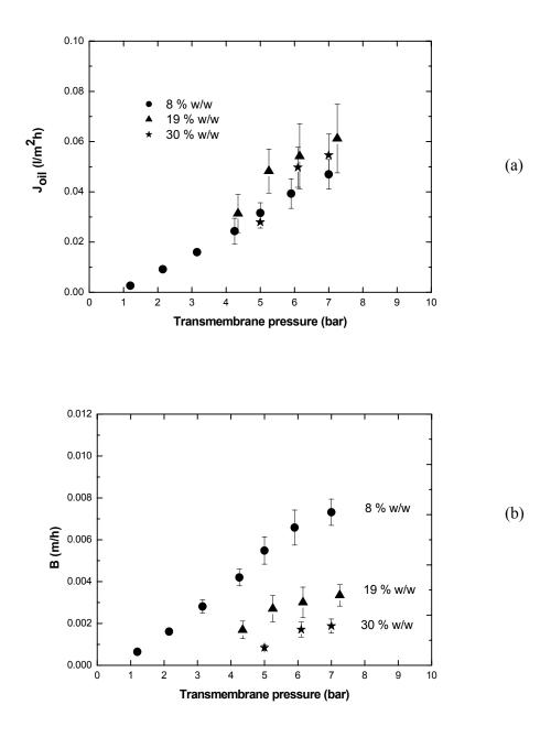
**Figure 6:** Effect of the transmembrane pressure upon (a) oil flux,  $J_{oil}$  and (b) oil permeability coefficient, B, for various oil/hexane concentrations.
