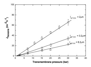
**Figure II.3:** Hexane flux as a function of transmembrane pressure through *PAN/PDMS* membranes of various effective thicknesses. Experimental conditions: 8% w/w oil/hexane feed, at  $24 \pm 3$  °C.
