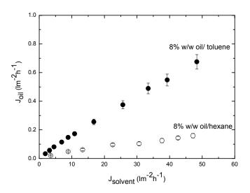
*Figure* 7: *Oil flux as a function of the solvent flux at feed concentration of 8 % w/w.*
