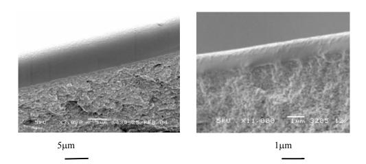
**Figure II.1:** Typical examples of the SEM images of cross-section of the prepared PAN/PDMS membranes with thicknesses of about: (a) 7 µm and (b) 1 µm.
