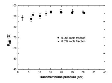
*Figure 15: Oil retention for the GKSS membrane as a function of transmembrane pressure, at various oil/hexane feed concentration, at 24 \pm 3 °C.*
