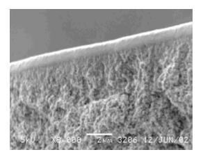
*Figure 1*: *SEM picture of the cross section of the M7-30, PAN/PDMS composite membrane.*
