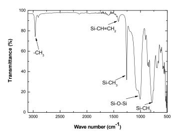
*Figure 3*: *ATR-FTIR spectra of the PDMS membrane prepared at ratio of 10/1.*
