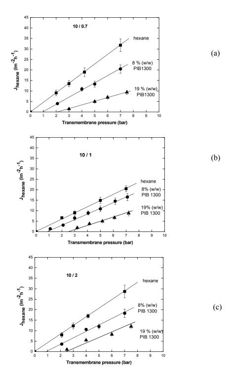
*Figure 11*: Hexane flux through PAN/PDMS membrane prepared at prepolymer/cross-linker ratios of (a) 10/0.7, (b) 10/1 and (c) 10/2 as a function of transmembrane pressure for various PIB 1300/hexane feed concentrations.
