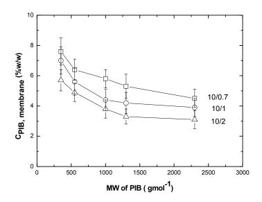
**Figure 7:** The effect of MW of PIB on the concentration of PIB/hexane solution inside the PDMS dense membrane prepared at pre-polymer/cross-linker of various ratios.
