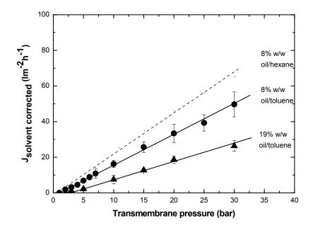
**Figure 6:** Corrected solvent flux through PAN/PDMS composite membrane as a function of transmembrane pressure for various oil/solvent concentrations, at  $24 \pm 3$  °C.
