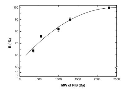
*Figure 9*: *PIB retention by the PAN/PDMS composite membrane as a function of the molecular weight of PIB. Feed concentration:* 8 % (*w/w*),  $\Delta p = 7$  bar at 24 ± 3 °C.
