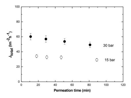
*Figure 5*: Total flux through PAN/PDMS membranes as a function of permeation time, at 0.008 mol fraction oil/hexane and  $24 \pm 3$  °C.
