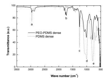
Figure 3: FTIR spectra of the dense PEO-PDMS-PEO and PDMS membranes.
