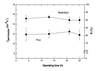
*Figure 10:* Permeate flux and oil retention of the M7-30. Experimental conditions: 7 bar, at  $24 \pm 3 \,^{\circ}$ C.
