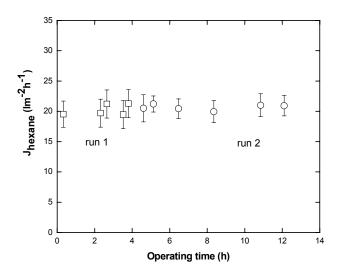
*Figure 9:* Hexane flux through the M7-30 composite membranes as a function of operating time. Experimental conditions: 7 bar,  $24 \pm 3 \,^{\circ}$ C.
