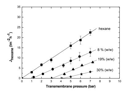
*Figure 4*: *Hexane flux as a function of transmembrane pressure for various oil/hexane feed concentrations.*
