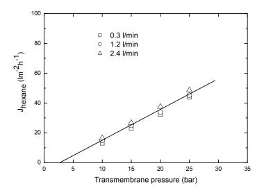
**Figure 8:** Hexane flux through the PAN/PDMS membrane as a function of transmembrane pressure, at various flow rates. Experimental conditions: concentration of 0.022 mol fraction, 25  $^{\circ}$ C.
