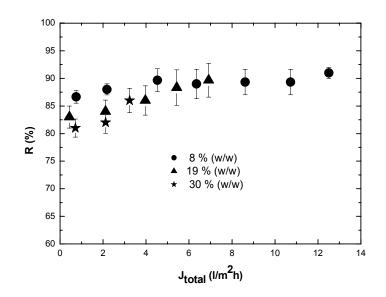
*Figure 8:* Oil retention by the PAN/PDMS composite membrane as a function of total permeate flux, for various oil/hexane concentrations.
