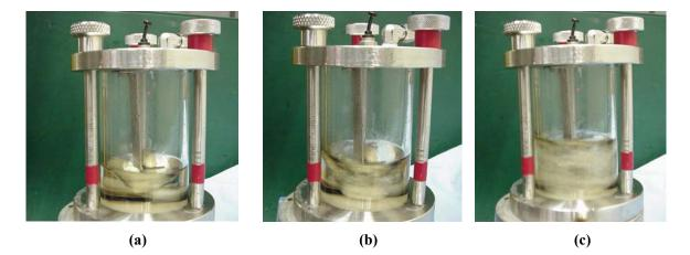
*Figure I.2*: Visualization of the vortex due to the stirring rate: (a) 300 rpm, (b) 700 rpm (c) 1400 rpm.
