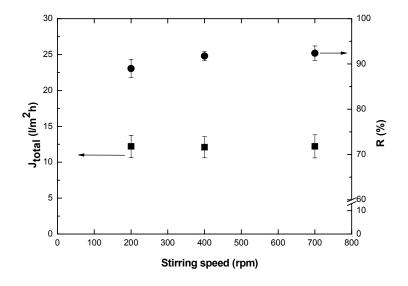
*Figure 3:* Effect of the stirring speed upon total permeate flux and retention of 8%(w/w) oil/hexane solution, at  $\Delta p = 7$  bar and  $24 \pm 3$ °C.
