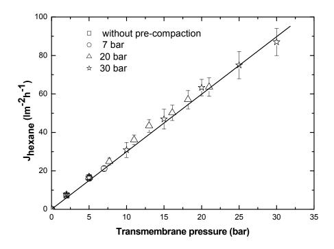
*Figure 3:* Hexane flux as a function of transmembrane pressure after various precompaction pressures, at  $24 \pm 3$  °C.
