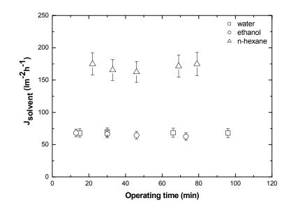
*Figure 5*: Solvent flux as a function of operating time through PAN support. Experimental conditions: transmembrane pressure of 1 bar, at  $24 \pm 3$  °C.
