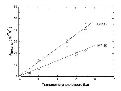
*Figure 15:* Hexane flux as a function of the transmembrane pressure, at  $24 \pm 3$  °C.
