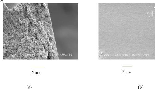
*Figure 4*: *SEM pictures of PAN support (a) cross section (magnification 4000x) and (b) surface (magnification 8000x).*
