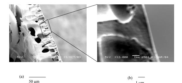
Figure 11: SEM pictures of the cross-section of MPF-50 membrane, (a) magnification of 500x and (b) zooming in (magnification 12000x) on details of the surface region.
