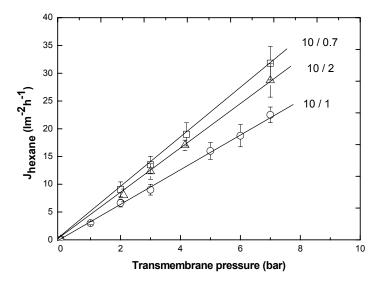
*Figure 9:* Hexane flux as a function of the transmembrane pressure for the *PAN/PDMS* membranes prepared at various pre-polymer/cross-linker ratios.
