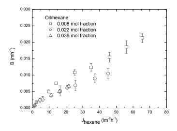
*Figure 11: Effect of the hexane flux upon oil permeability coefficient, at various oil/hexane concentrations.*
