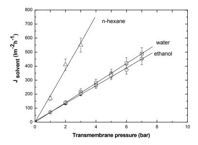
*Figure 6*: Solvent flux as a function of transmembrane pressure, at  $24 \pm 3$  °C.
