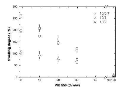
*Figure 6:* The effect of the solution concentration upon swelling degree of the *PDMS* dense membranes prepared at pre-polymer/cross-linker of various ratios.
