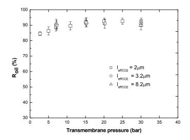
**Figure II.4:** Oil retention by the PAN/PDMS composite membrane as a function of transmembrane pressure and effective thickness. Experimental conditions: 8 % w/w oil/hexane solution, at  $24 \pm 3$  °C.
