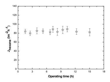
*Figure 2*: Hexane flux through PAN/PDMS membrane as a function of operating time, at 30 bar and  $24 \pm 3$  °C.
