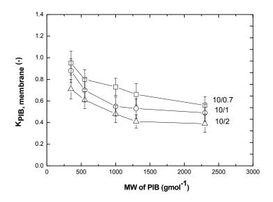
*Figure 8:* The PIB partition coefficient for the PDMS dense membranes prepared at pre-polymer/cross-linker of various ratios.
