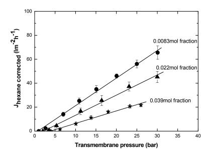
*Figure 7:* The hexane flux through PAN/PDMS membrane as a function of transmembrane pressure, at various oil/hexane concentrations and  $24 \pm 3$  °C.
