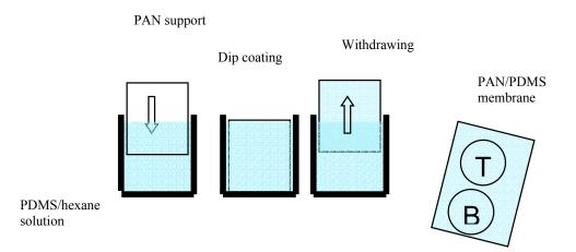
*Figure 2*: Schematic drawing of the dip coating process (*T* and *B* indicates the top and bottom side, respectively, of the PAN/PDMS composite membrane).
