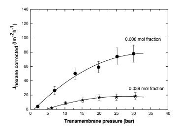
*Figure 14:* The hexane flux through GKSS membrane as a function of transmembrane pressure, at various oil/hexane concentrations and  $24 \pm 3 \,^{\circ}$ C.
