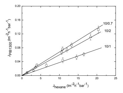
*Figure 12: The flux of PIB 1300 as a function of the hexane flux for various crosslinking degrees of PDMS. Feed concentration: 8 % (w/w).*
