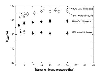
*Figure 9:* Oil retention by the PAN/PDMS composite membrane as a function of transmembrane pressure, for 8 and 19% (w/w) oil/toluene and oil/hexane solutions.
