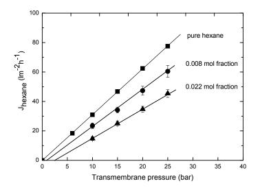
*Figure 9:* Hexane flux through the PAN/PDMS membrane as a function of transmembrane pressure, at various oil/hexane concentrations and 25 °C.
