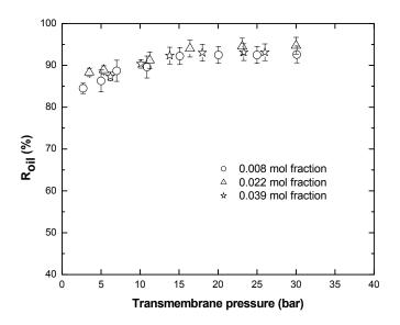
*Figure 10:* Oil retention by PAN/PDMS membrane as a function of transmembrane pressure, at various oil/hexane concentrations and  $24 \pm 3$  °C.
